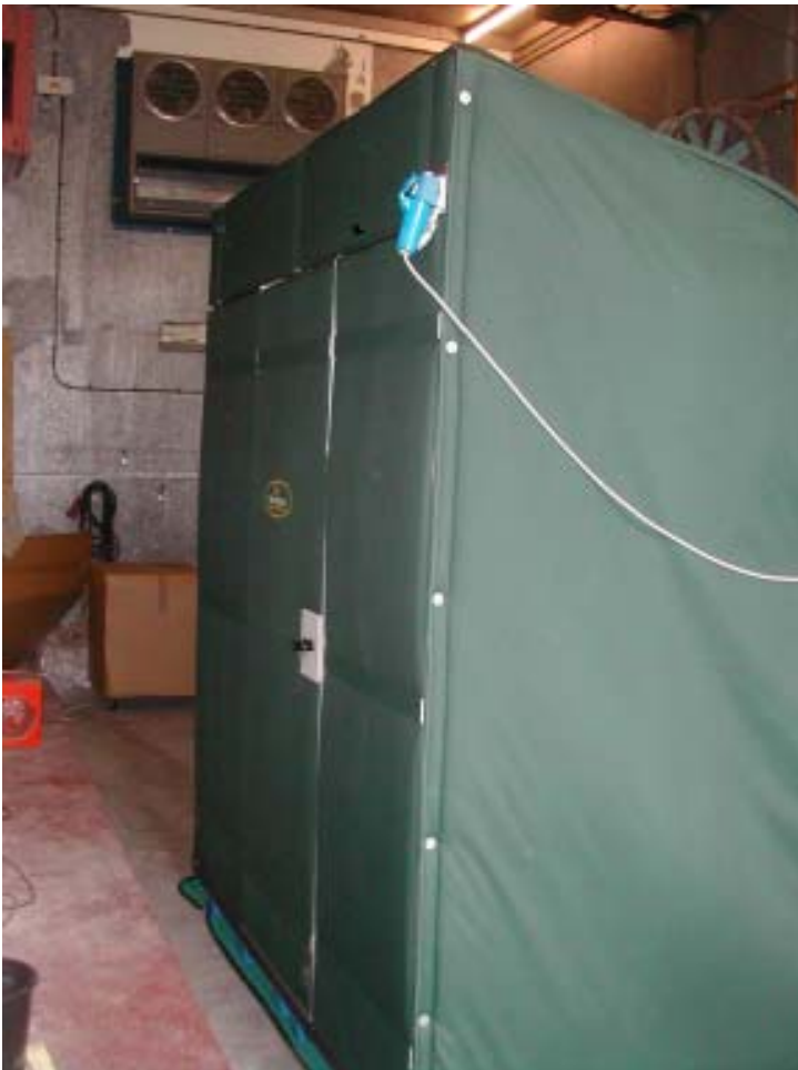
Figure 4 – Front Photograph of the Cold Store set up in Test Chamber 1
